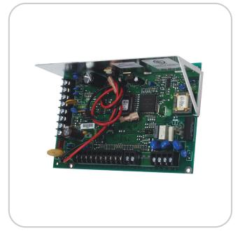
Control panel with 6 points and full data interface to UPLINK Model 1600 Cellular/Cellemetry Radio Transceiver.
